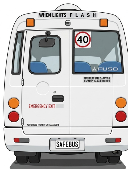
Fig. 3 — Rear decal placement, rear doors
