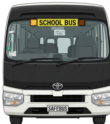
Fig. 3 — Sign & lights fitted, front view
