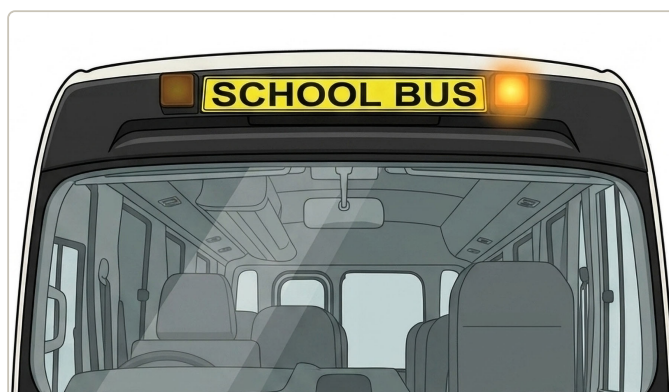
Fig. 3 — Sign & lights fitted, front view
