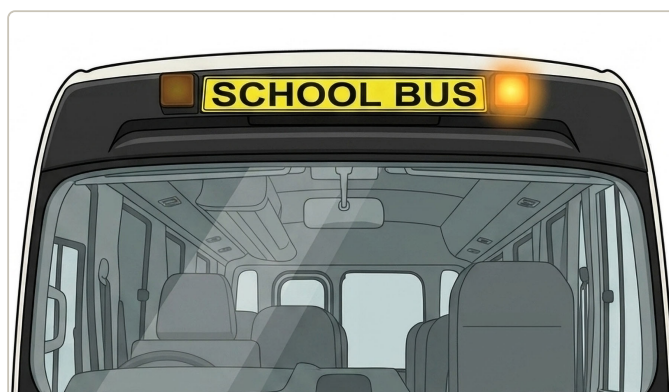
Fig. 3 — Sign & lights fitted, front view
