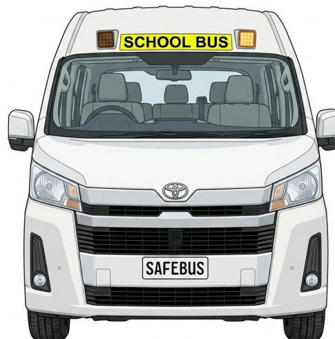
Fig. 2 — Sign & lights fitted, front view
