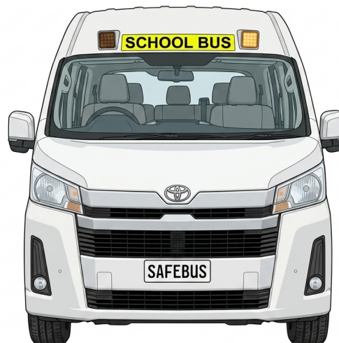
Fig. 2 — Sign & lights fitted, front view
