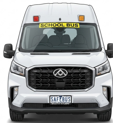
Fig. 2 — Sign & lights fitted, front view
