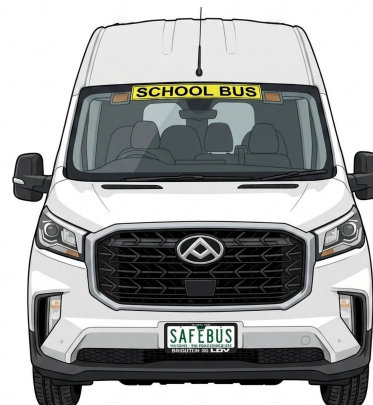
Fig. 2 — Sign & lights fitted, front view
